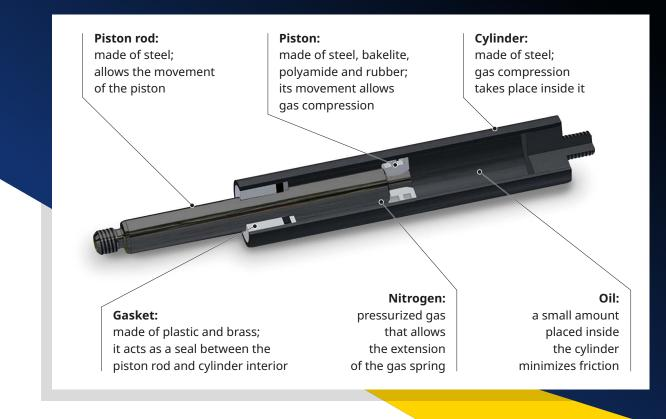
The gas spring works by compressing the pressurized nitrogen inside the cylinder. This happens when the piston rod is pushed by the weight of the tailgate (or the car hood) inside the cylinder, pushing the piston itself and compressing the gas, providing the so-called 'extension force' when the tailgate is reopened.
